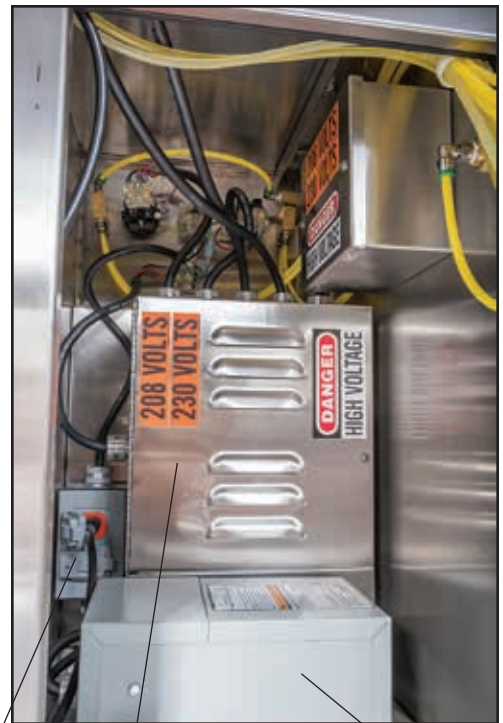
Fig. 44 110V Outlet Box Control Box Transformer
